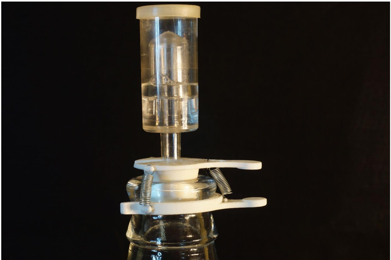
Assembled retainer clip holding a stopper and airlock in the mouth of a 3-gallon glass carboy.
